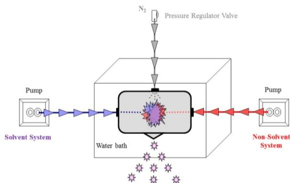
**Figure 1 Schematic representation of MJR experimental set-up:** Solvent and non-solvent were delivered to the MJR at equal flow rates at 180° angle. NPs were collected from the bottom opening of MJR. The system was immersed in a water bath in order to control the overall temperature.
