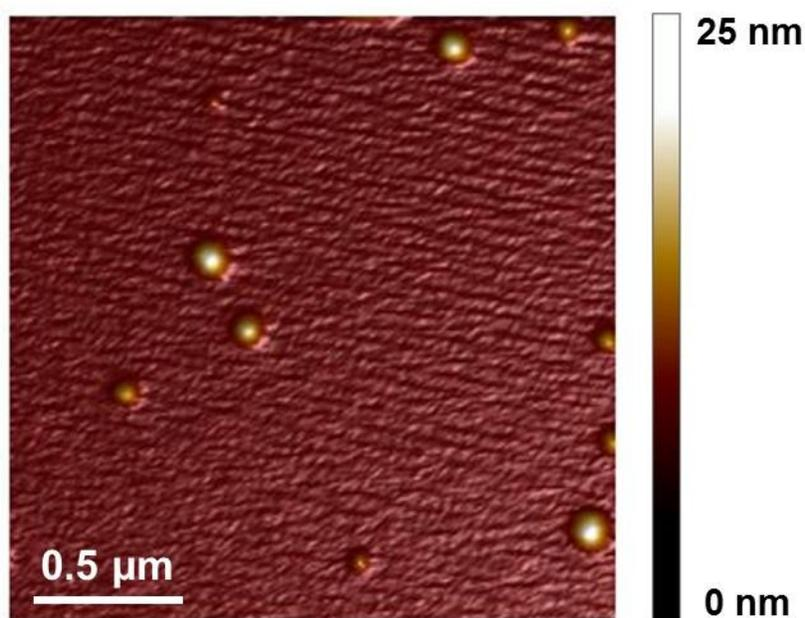
**Figure 2: Complex-loaded nanoparticle morphology:** Atomic force microscopy revealed spherical shape with smooth surface
